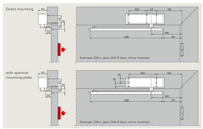
Depending on construction conditions, the door opening angle is limited to approx. 120° to 145°. To prevent damage to the door and door closer, we recommend using the opening restrictor or placing a door stop.
