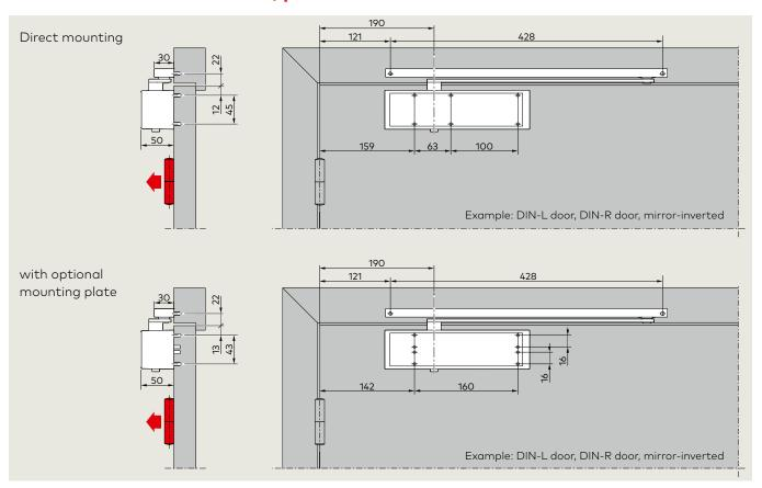
A  $180^{\circ}$  opening angle is possible in this installation type, provided that the appropriate construction conditions are met. In most cases, the door closer requires a wall recess for that purpose.
